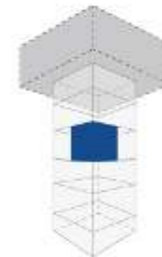
普通货物的机房 Machine room in the ordinary elevator
