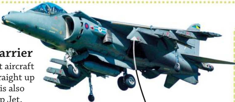
Downward-facing engines help the plane take off.
