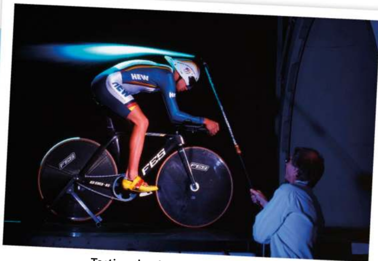
Testing the design of an Olympic bicycle in a wind tunnel
