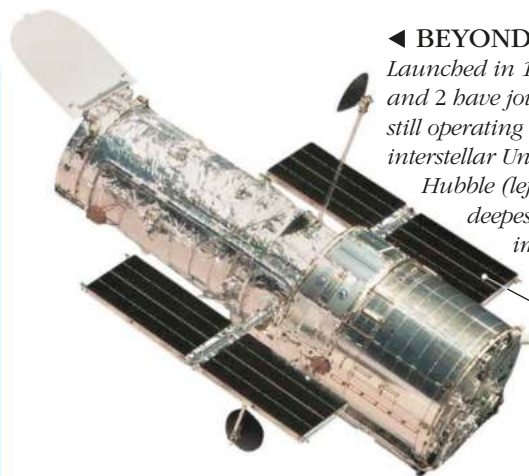
The 7.6 m (25 ft) long solar panels generate power from the Sun.
